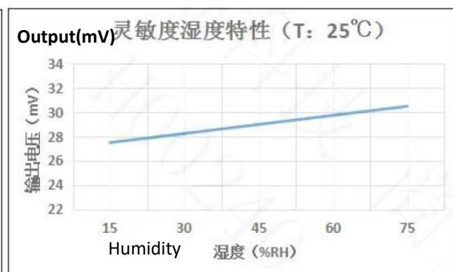
Fig8. Sensitivity at different humidity
