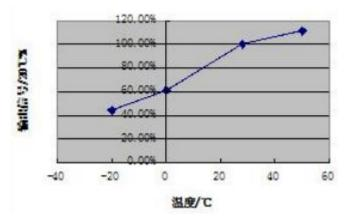
(4) Zero point output in different temperature
